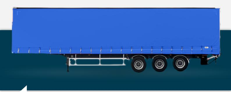
The curtainside trailer combines the benefits of a flatbed with the covering and containment advantages of an enclosed trailer. At ADAA TENTS, SHEDS & TARPAULINS TRADING CO. L.L.C., we specialize in providing high-quality Curtain side for your trailer. Our side Curtain are made of durable PVC 900GSM Heavy Duty PVC Tarpaulin side curtains, retractable from either the front or rear of the trailer.
